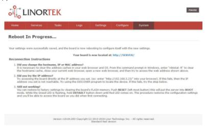
Note: you can also enter the bootloader mode by pressing the RESET switch on your SERVER.
